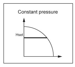
The pump maintains a constant pressure at any flow demand. The desired head of the pump can be set via user interface.
