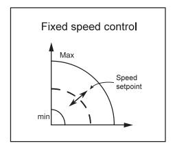
The pump maintains a fixed speed at any flow demand. The speed of the pump can be set via user interface. Constant speed is great when used in the primary or boiler loop in a primary/secondary hydronic system.
