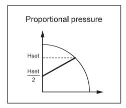
The pump pressure is continuously increased / decreased depending on the flow demand. The maximum head can be set via user interface.
