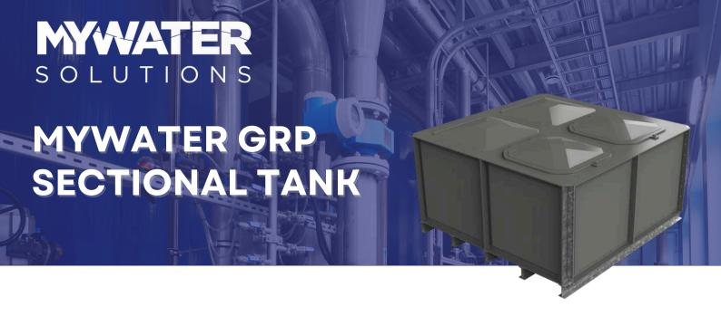
The GRP Sectional Hot Press Moulded Tanks are modular water storage solutions designed for large-capacity applications, ranging from 125 litres to 2 million litres. Manufactured using hot press moulded GRP panels, they ensure maximum dimensional stability, durability, and compliance with WRAS and BS EN 13280:2001 standards.
